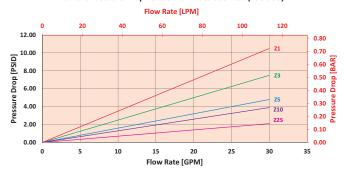
$$\triangle P_{\text{filter}} = \triangle P_{\text{housing}} + (\triangle P_{\text{element}} * \forall_f)$$
