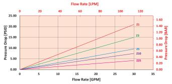
2AZ Element Pressure Drop versus Flow Rate at 32 cSt (150 SUS)
