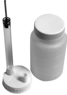
The Probalizer Sampling Test Point provides a point of access for obtaining representative fluid samples from an operational hydraulic system. The downstream channel is specially sized to accept the sampling probe from a customized cap/probe assembly screwed onto a sample bottle. (See photo). Use of this system minimizes leakage and helps to maintain the integrity of the sample.
