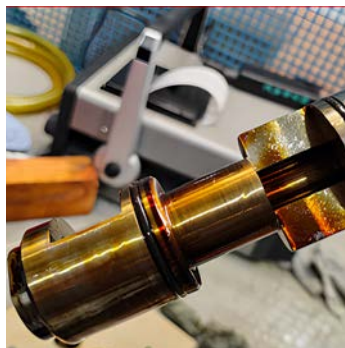
Varnish deposits on hydraulic valve component
