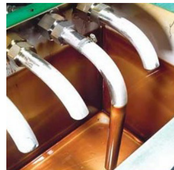
Varnish layer on reservoir interior walls
