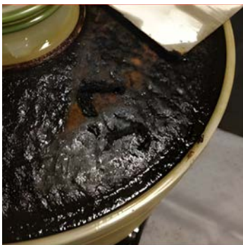
Varnish buildup on a filter element
