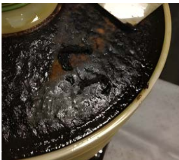
Varnish buildup on a filter element
