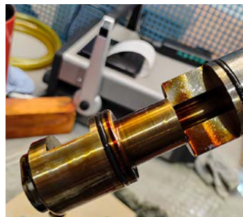
Varnish layer on hydraulic valve component
