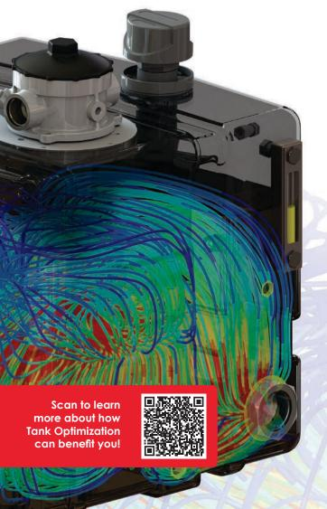
The goal of hydraulic tank optimization is to reduce the reservoir size and thus reduce its fluid volume. Two primary factors determine how much a tank can be optimized:
