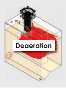
Removing air from the hydraulic fluid is one of the most important roles of the hydraulic tank and return-line filter.
