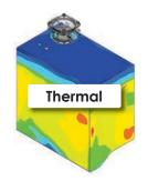
Temperature reveals a lot about the quality of a reservoir design. How quickly/evenly does the fluid reach operating temperature? Could hot spots be indicating faster fluid degradation? Do cold spots signify stagnant flow? Thermal simulations provide these valuable insights!
