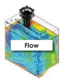
Flow simulations assess the flow patterns and velocity of fluid within the tank. Fast, turbulent flow can lead to air contamination or poor de-aeration. Stagnant pockets in the reservoir indicate inefficient circulation and wasted space.
