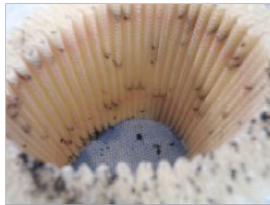
Photo 2 Holes in glass media and discoloration caused by electrostatic discharge.
