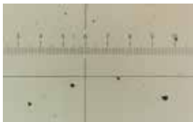
ISO 18/16/13 NAS 1638: Class 7 SAE AS 4059(D): Class 8
