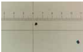
ISO 16/14/11 NAS 1638: Class 5 SAE AS 4059(D): Class 6
