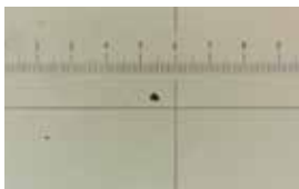
ISO 15/13/10 NAS 1638: Class 4 SAE AS 4059(D): Class 5
