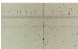
ISO 21/19/16 NAS 1638: Class 10 SAE AS 4059(D): Class 11
