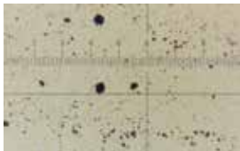
ISO 22/20/17 NAS 1638: Class 11 SAE AS 4059(D): Class 12
