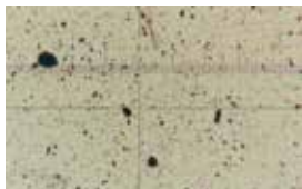
ISO 23/21/18 NAS 1638: Class 12 SAE AS 4059(D): Class 13
