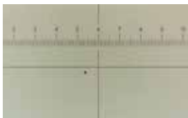
ISO 14/12/9 NAS 1638: Class 3 SAE AS 4059(D): Class 4
