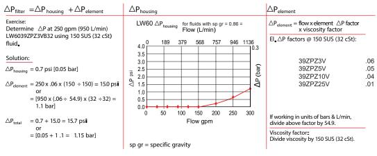
Sizing of elements should be based on element flow information provided in the Element Selection chart above. Please note that 95/5 fluid has a lower viscosity than 150 SUS and therefore pressure drops for 95/5 will actually be lower.
