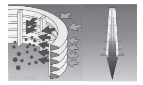
The backflush valve opens and closes during backflushing of each filter element, further minimizing the amount of filtrate needed to effectively clean the element.
