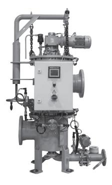
The AutoFilt® RF14 is a self-cleaning system for extracting particles from low viscosity fluids. Its robust construction and automatic back-flushing capability make a major contribution to operational reliability and reduce operating and maintenance costs. The slotted or SuperMesh baskets in the filter with filtration rates from 10 to 100µm ensure highly effective filtration of contaminating particles from the process medium.
