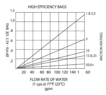
**Step 1** The graphs show the  $\triangle$ PB produced by a #2 size bag for water, 1 cps @ 77°F (25°C). The pressure drop is determined from the type of bag, the micron rating and flow rate.
