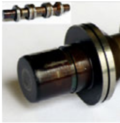
Valve piston with deposits
