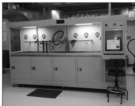
Fluid Care Center: Multi-Pass Test Stand
