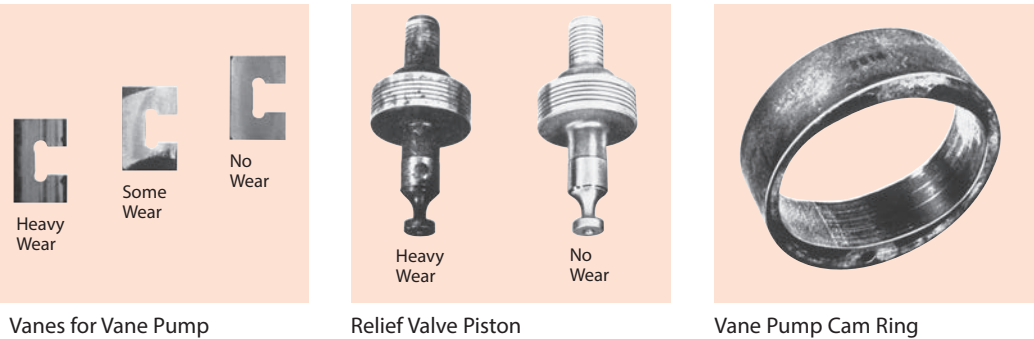
Figure 1. Typical Examples of Wear Due to Contamination
