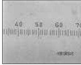
Figure 31. Cleanliness Class Achieved by the Test Fluid: NAS 3
