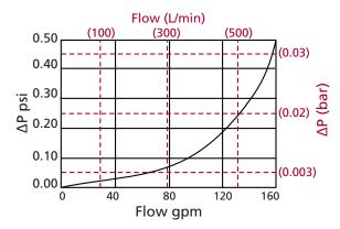
**Pressure** Drop Information Based on Flow Rate and Viscosity
